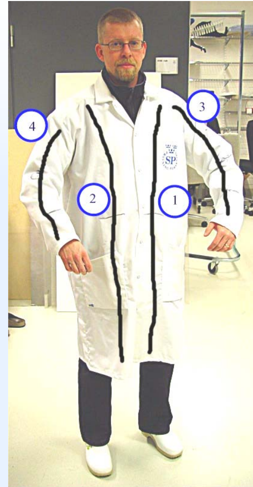
ESD protective garment with indicated measurements paths
